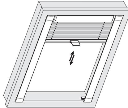
Attach the control rod to the operating handle (option).
