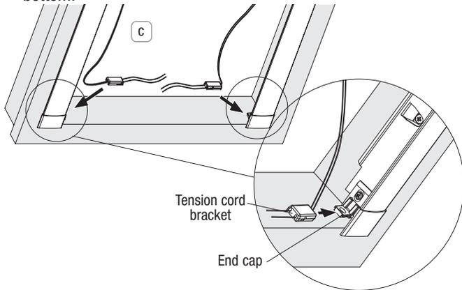
After having checked that the pleated blind functions as prescribed, the excess cord ends can be cut off.
