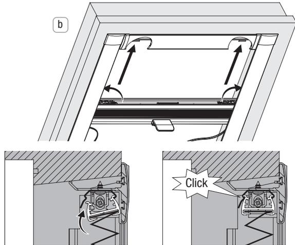
d) Push the tension cord brackets over the end caps at the bottom.
