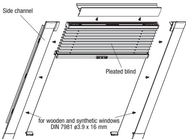
**Information:** The older window model GGU with 105° mortise requires the spacers supplied to be inserted into the running rail. Place the spacers near the screw.
