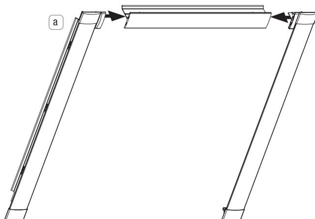
b) Put the profiles into the window frame. The top profile must fit tightly at the top.
