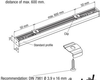
b) Depending on the window type and brand the distance to the front edge of the window is determined by use of the mounting template. Mark up the drilling holes by use of a pin and fix the clips with the screws.
