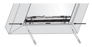
b) Push the fixing plate into the mounting template.
