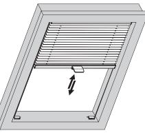
Attach the control rod to the operating handle.
