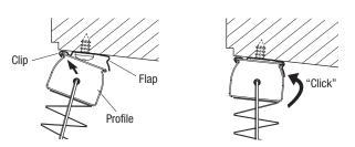
When **dismounting**, push the flap of the clip upwards to be able to take the profile out of the clip.
