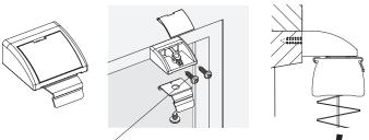
Recommendation: DIŃ 7981 Ø 2,9 x 9,5 mm (for wooden and synthetic frames)
