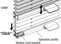
After having checked that the pleated blind functions as prescribed, the excess cord ends can be cut off.
