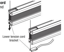
Installing the window moulding with moulding locking strip
