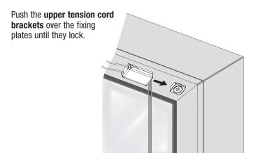
Take the lower tension cord brackets out of the rail and push them over the fixing plates until they lock.
