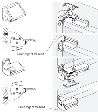
Recommendation: DIN 7981 Ø 2.9 x 9.5 mm (for wooden and synthetic frames) Max. length of the screw = window moulding depth!
