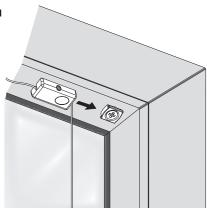
Take the lower tension cord brackets out of the rail and push them over the fixing plates until they lock.
