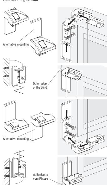
Recommendation: DIN 7982 Ø 3.9 x 13 mm (for wooden and synthetic frames)
