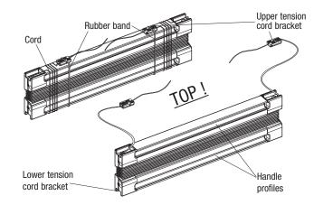
Push the upper tension cord brackets over the fixing plates until they lock.
