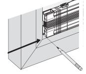
**Mounting glass border** with fixing plates
