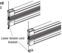
Installing the window moulding with moulding locking strip
