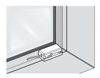
Glass strip mounting with attachment bracket (edge)
