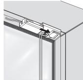
Take the **lower tension cord brackets** out of the rail and push them over the fixing plates until they lock.
