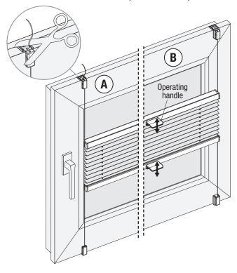
Attention: Adjustment of the cord tension must be uniform and may only be made by a professional!
